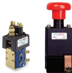
The **DC Contactor SW80** is rated for 100 amps in severe switching applications and 125 amps in light-duty switching applications.
