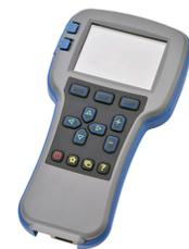
**The Curtis Model 1313 Handheld Programmer** is ideal for setting parameters and performing diagnostic functions.
